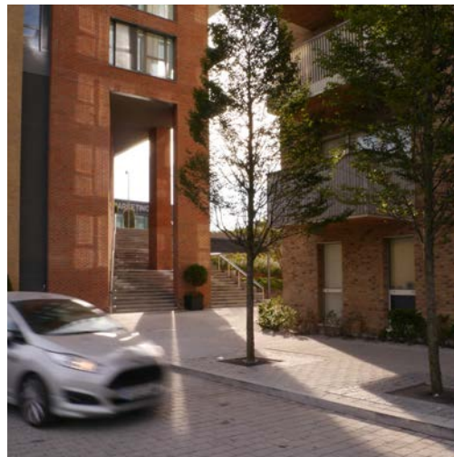
St Andrews in Bromley-By-Bow uses shared surface treatment for the smaller roads between the new residential blocks
